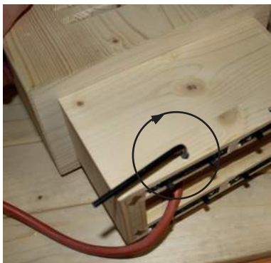
Fig. 28: Attach the front radiator in place
