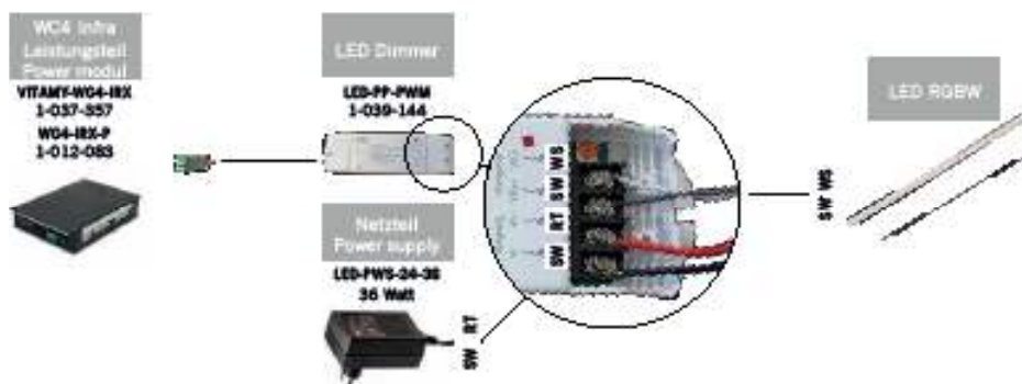
Fig. 27: Connecting the LED RGBW to the control unit
